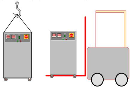
**Note:** Floor Mounted Dryers can be lifted by hoist or fork lift.
